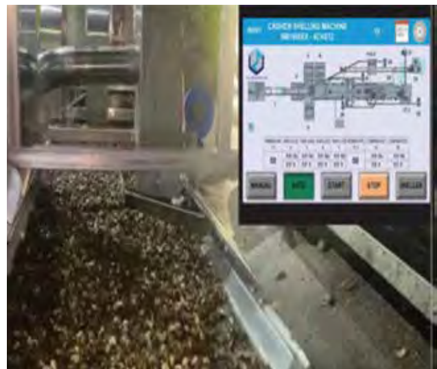
Separating cashew kernels from machine and oil-contamination agents
